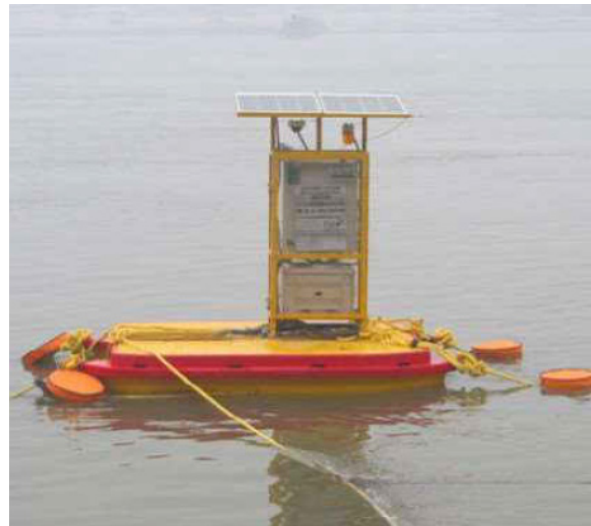
Figure 3: Floating type real-time water quality monitoring station
